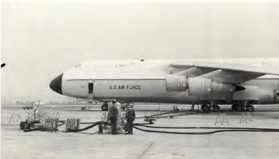
Refueling—C-5A can be fueled at rate of 2400 gallons per minute through four single point receptacles with 600 gpm rate each.
