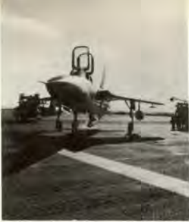
Air Force fire fighters approach an F-105 Thunderchief which developed hot brakes during landing. U. S. AIR FORCE PHOTO, Det. 5, HQ AAVS.
